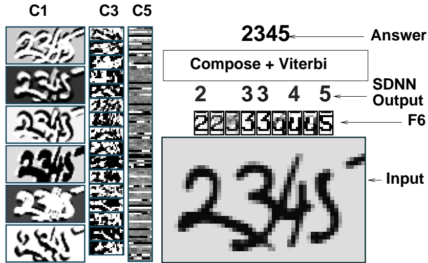
Fig. 6. An example of multiple character recognition with SDNN. With SDNN, no explicit segmentation is performed.
