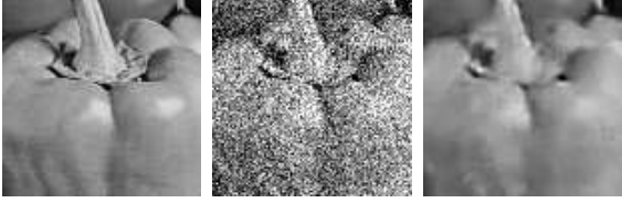
Figure 4: Example of denoising (details of the “peppers” image). Left panel: original image. Central panel: noisy image ( \sigma = 50 ); PSNR equal to 14.15dB. Right panel: reconstructed image using a machine trained to reconstruct clean patches from noisy ones (with \sigma = 50 ); PSNR equal to 26.35dB.
