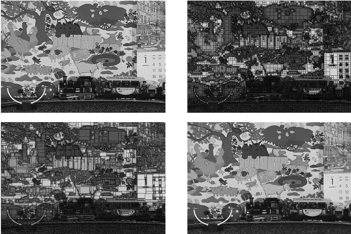
Figure 2: Effects of boxletization: original (top left), greedy (bottom left) with a threshold of 10,000, and recursive (top and bottom right) with a threshold of 10,000.
